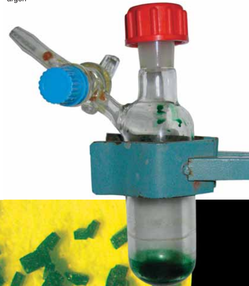
This is how the dark green \text{Cs}_4\text{Ta}_6\text{Br}_{12}(\text{NCS})_6 \cdot 0,5\text{H}_2\text{O} crystals look
