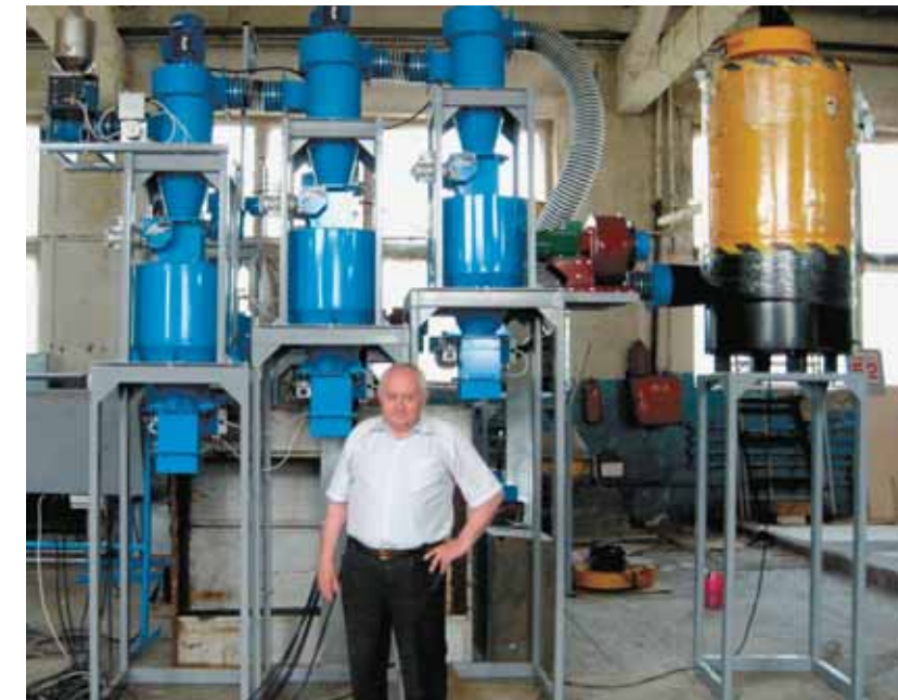
Main components of a pilot plant for mechanochemical processing of vegetable feedstock (productivity 100 kg/h): mill-activator and separator for feedstock enrichment. Design of ISSCM, SB RAS (Novosibirsk)
