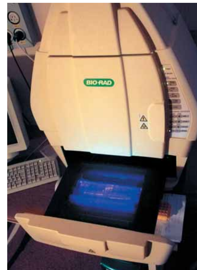
Transilluminator is designed to detect the fragments of nucleic acids in ultraviolet
