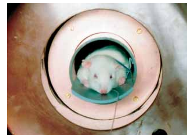
A laboratory rat in the resonator of EPR-spectrometer in the experiment of pH monitoring in a stomach
