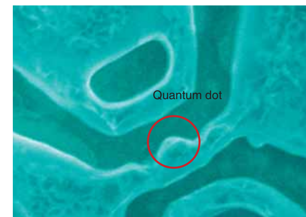
Image of the new single-electron transistor under an electronic microscope. Picture by A. Plotnikov
