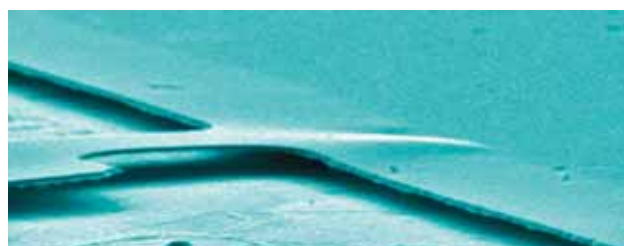
The conductive semiconductor membrane 110 nm thick is "suspended" above the substrate at the height of 400 nm. The suspension is achieved by selective etching-out of the "sacrificial" layer under the upper working one. The method of making these membranes is well-known, but it has never been used to make nano-structural elements. Today, such structures are used at the Institute of Semiconductor Physics SB RAS as a basis for making the so-called "suspended" single-electron transistors. Electron microscopy. Picture by T. Gavrilova
